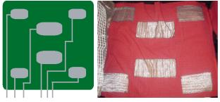
Figure 3. Final seat sensor layout sketch (left), prototype made out of conductive fabric and conductive thread (right)
