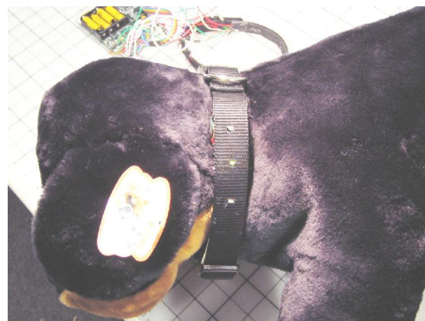
Figure 2: Top picture shows the collar with its modified UbER-Badge. Lower picture show how the collar fits on the stuffed dog.
