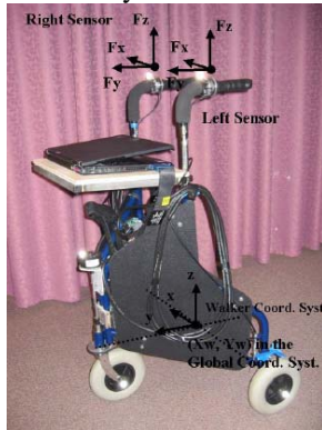
Figure 1. COOL Aide hardware configuration
