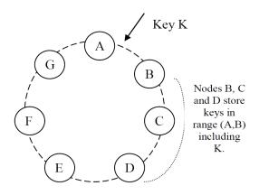
Figure 4.1.: Amazon's Dynamo – Consistent Hashing with Replication (taken from [DHJ<sup>+</sup>07, p. 209])
