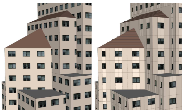
Figure 2: The motivation for our novel shape grammar. The modeled building consists of 14 volumetric primitives (cubes, roofs) placed by a stochastic shape grammar. Left: Existing methods of procedural architecture can either place shaders on the individual volumes or use split rules for procedural refinement. In both cases several unwanted intersections will cut windows (or other elements) in unnatural ways, as the volumes are not aware of each other. Right: Our approach allows the resolution of these conflicts. Additionally, we can place geometry on polygons of different orientation such as roof surfaces. This example was created using only 6 rules.
