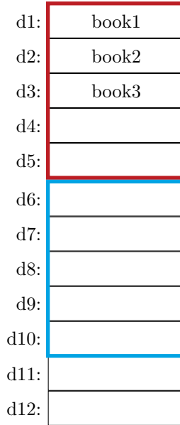
Figure 7.2: Our memory storage. Here, the red line indicates that we set aside 5 blocks for kids books, and the blue indicates that we set aside 5 blocks for other books.
