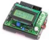
**Pololu Orangutan LV-168** [<http://www.pololu.com/catalog/product/775>]: a full-featured, mega168-based robot controller that includes an LCD display. The LV-168 runs on an input voltage of 2-5V, allowing two or three batteries to power a robot.
