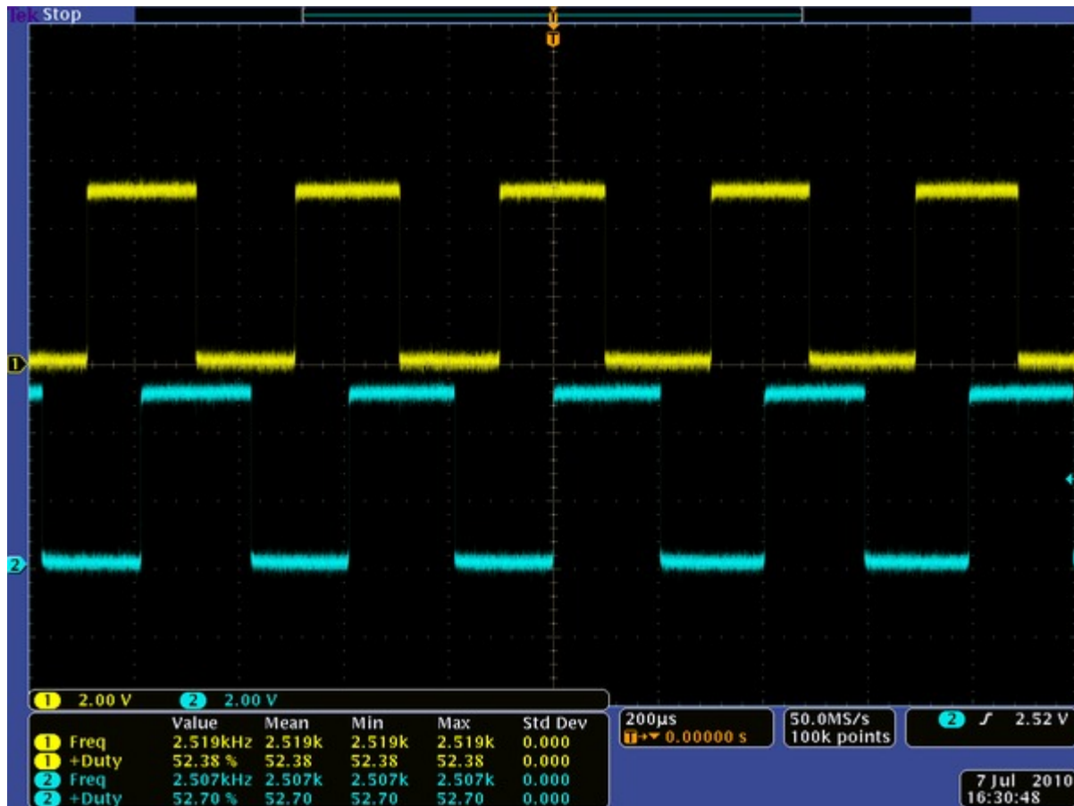
Encoder A and B outputs for 37D mm metal gearmotor with 64 CPR encoder (motor running at 12 V).
