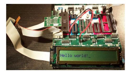
Figure 9: Wiring of the STK500
