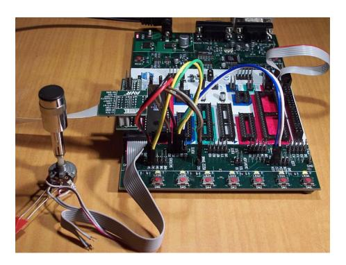
Figure 6: Setup of the STK500
