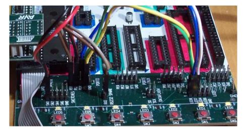
Figure 8: Wiring option #2 of the STK500
