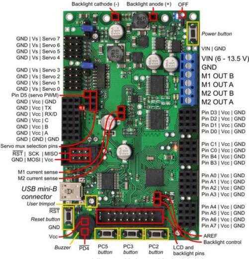
Orangutan SVP fully assembled PCB with pins labeled.
