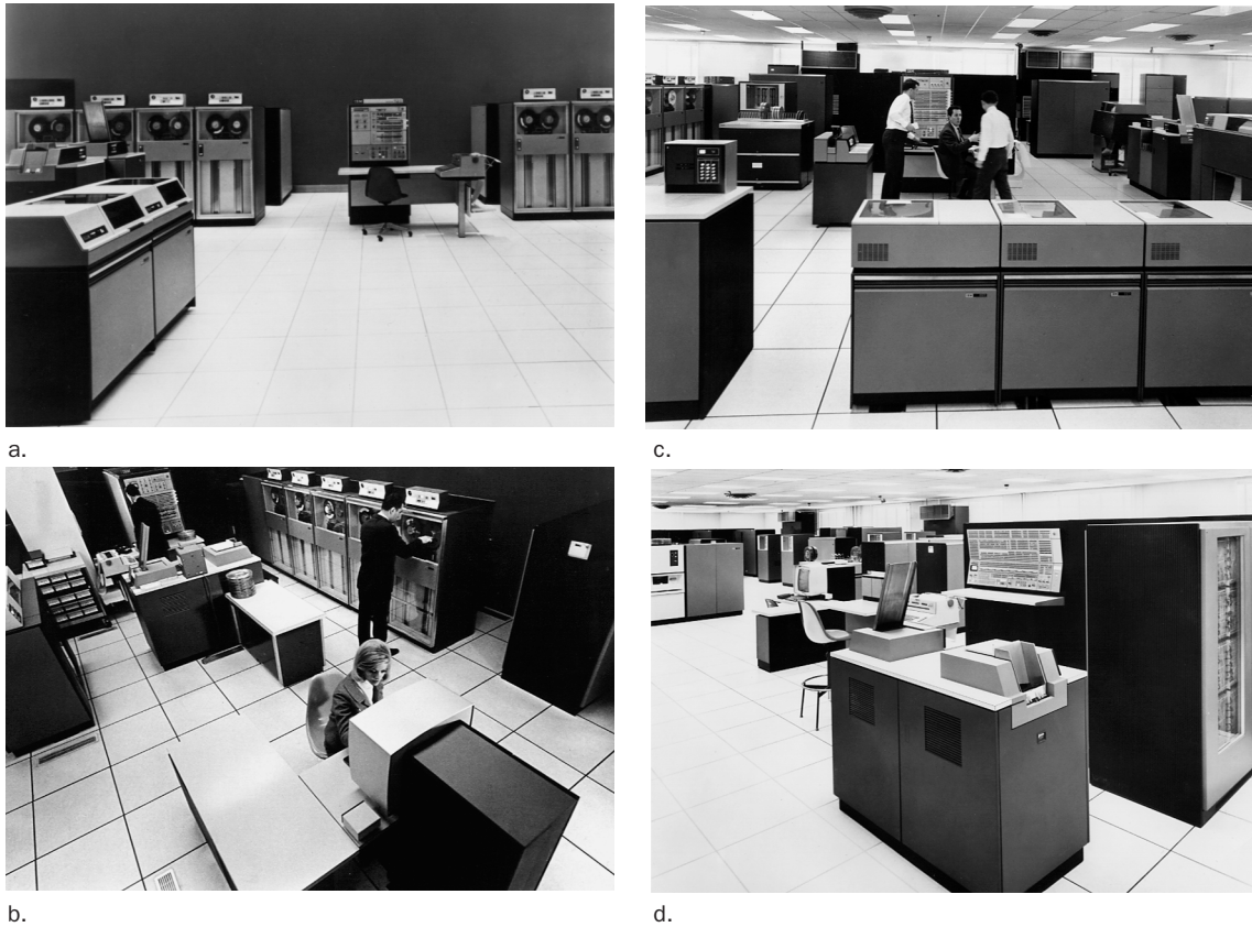
FIGURE 1.7.3 IBM System/360 computers: models 40, 50, 65, and 75 were all introduced in 1964. These four models varied in cost and performance by a factor of almost 10; it grows to 25 if we include models 20 and 30 (not shown). The clock rate, range of memory sizes, and approximate price for only the processor and memory of average size: (a) Model 40, 1.6 MHz, 32 KB–256 KB, $225,000; (b) Model 50, 2.0 MHz, 128 KB–256 KB, $550,000; (c) Model 65, 5.0 MHz, 256 KB–1 MB, $1,200,000; and (d) Model 75, 5.1 MHz, 256 KB–1 MB, $1,900,000. Adding I/O devices typically increased the price by factors of 1.8 to 3.5, with higher factors for cheaper models.
