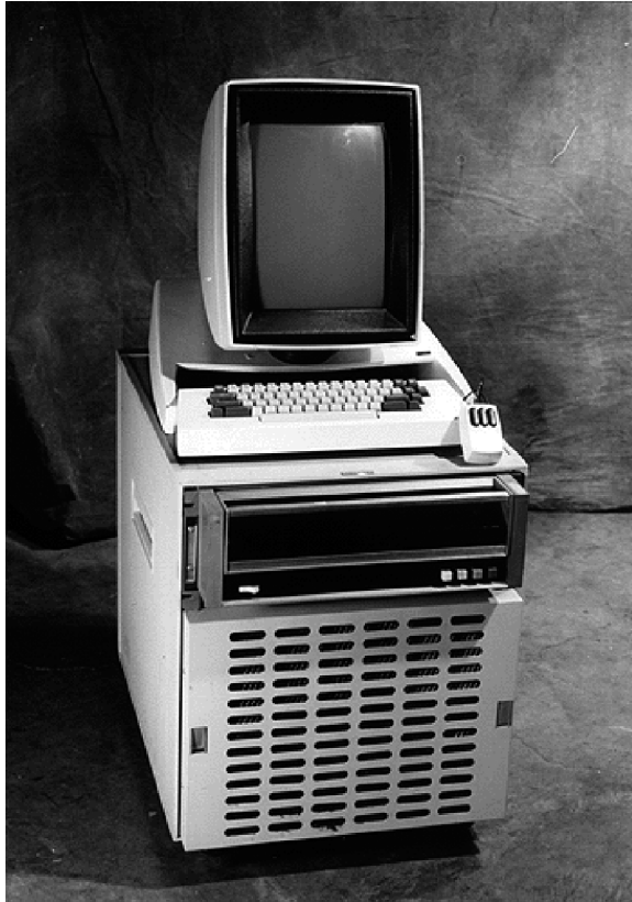
FIGURE 1.7.6 The Xerox Alto was the primary inspiration for the modern desktop computer. It included a mouse, a bit-mapped scheme, a windows-based user interface, and a local network connection.
