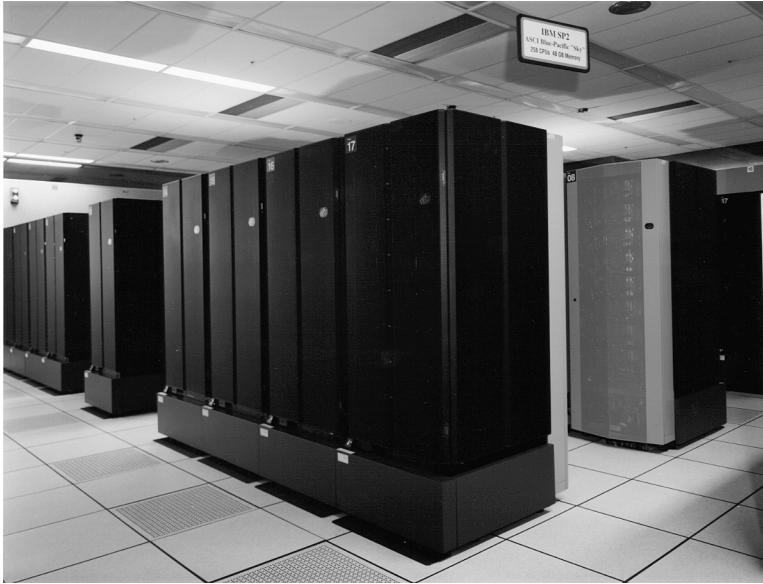
FIGURE 9.11.4 The IBM RS/6000 SP2 with 256 processors. This distributed-memory machine is built using boards from desktop computers largely unchanged plus a custom switch as the interconnect. In contrast to the SP2, most clusters use an off-the-shelf, switched local area network. Photo courtesy of the Lawrence Livermore National Laboratory.
