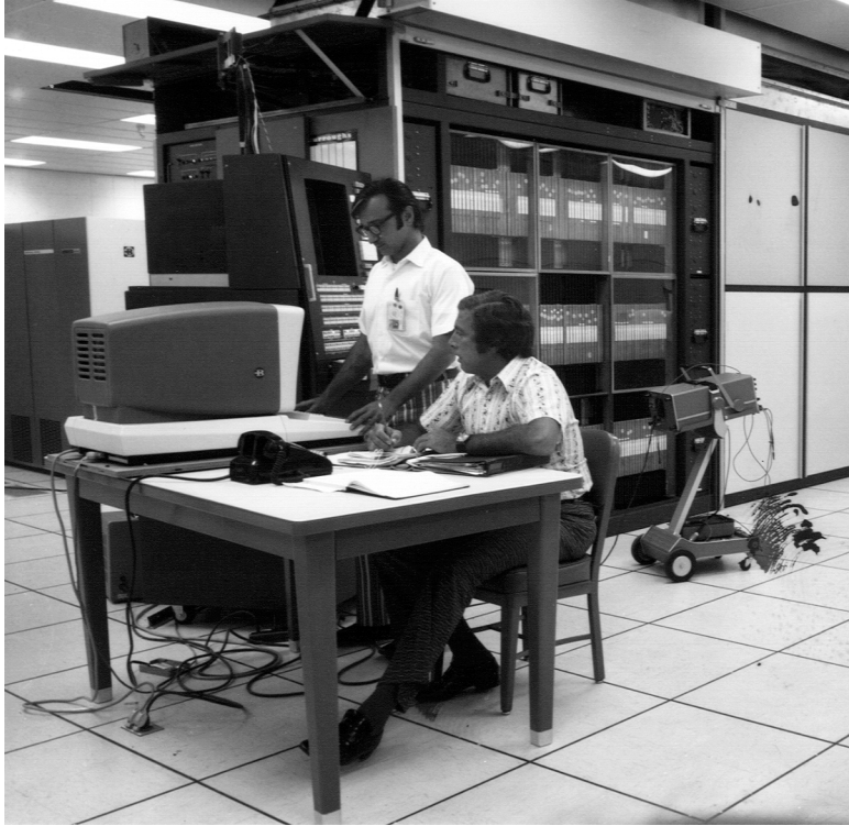
FIGURE 9.11.2 The Illiac IV control unit followed by its 64 processing elements. It was perhaps the most infamous of supercomputers. The project started in 1965 and ran its first real application in 1976. The 64 processors used a 13-MHz clock, and their combined main memory size was 1 MB: 64 \times 16 KB. The Illiac IV was the first machine to teach us that software for parallel machines dominates hardware issues. Photo courtesy of NASA Ames Research Center.
