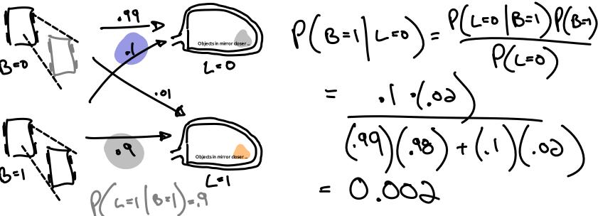
A blind spot monitor produces a warning light (L=1) when it estimates that a car is in one's blind spot (B=1). Given that the light is off, whats the probability that a car is one's blind spot? (Assume that a car is in your blindspot .02 of the time while driving.)
